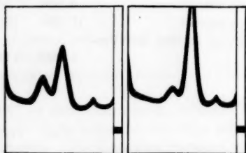
FIG. 2. Ultracentrifuge patterns of enzyme preparations with activities of 5620 and 8290 phosphatase units per mg. of protein nitrogen, respectively. Conditions of ultracentrifugation involved 1.2 and 1.5 mg. of protein nitrogen per ml., respectively; solvent, 0.01 M DL-alanine in 0.1 ionic strength phosphate buffer of pH 7.2; 70 minutes at 30°; 52,640 r.p.m. rotor speed.
